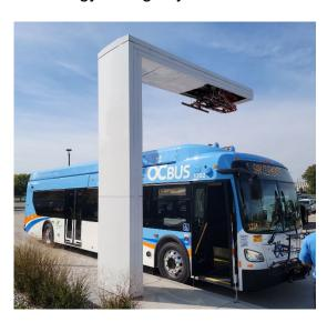
The existing rails mounted on the roof of the OCTA buses are based on New Flyer's configuration in accordance with SAEJ3105 charge rail positioning. The approximate location is shown in the images below.
